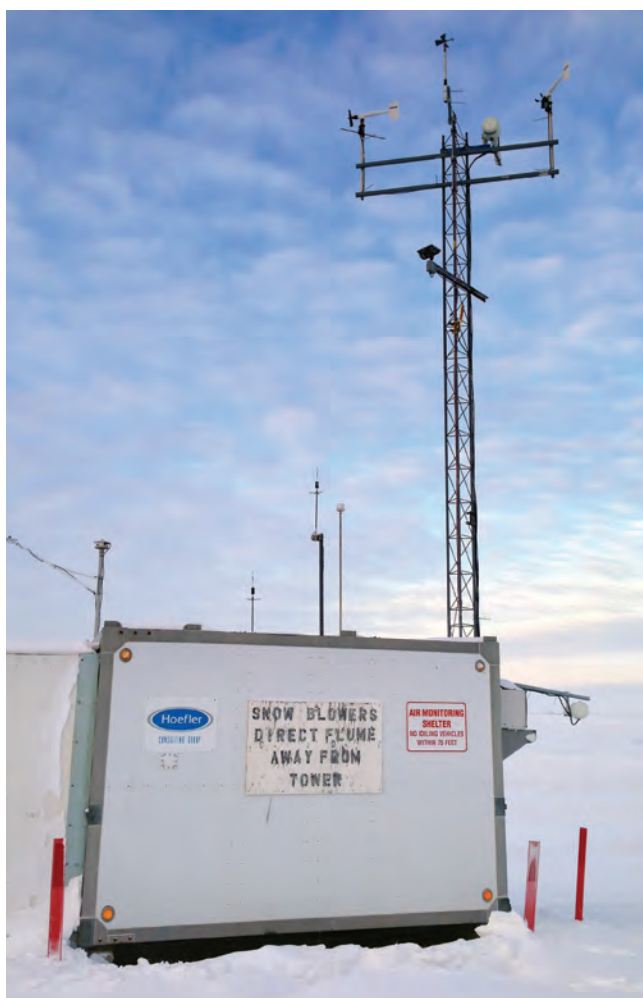
Figure 9-18. Ambient Air Monitoring Station on the North Slope (As the Arctic oil fields continue to mature, stations like this one could be maintained by a research and monitoring consortium.)
