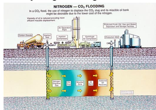
Figure 2: Illustration of the concept of EOR, where gas is pumped into the reservoir forcing oil to the production well. Source: DOE, NETL, at [http://www.netl.doe.gov/technologies/oil-gas/EP\\_Technologies/ExplorationTechnologies/eordraw.html](http://www.netl.doe.gov/technologies/oil-gas/EP_Technologies/ExplorationTechnologies/eordraw.html)
