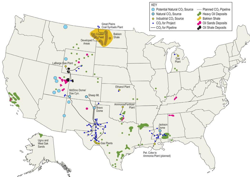
Figure 3. The current carbon dioxide EOR infrastructure, areas of development, and domestic oil resources in unconventional reservoirs, including the fractured Bakken shale of the Williston Basin. Source: DOE, National Energy Technology Laboratory, *Unconventional Fossil Energy Resource Program, Program Fact Sheet*, April 2011, [www.netl.doe.gov/publications/factsheets/program/Prog100.pdf](http://www.netl.doe.gov/publications/factsheets/program/Prog100.pdf).
