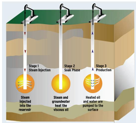
CSS performance is measured based on steam-oil-ratio<sup>60</sup> (SOR), well productivity, and overall recovery factor. Operating mature CSS projects reported average SORs of about 3.0-6.0 and average bitumen production rates of about 40-90 B/D per well in 2009.<sup>61</sup> Individual well pad
