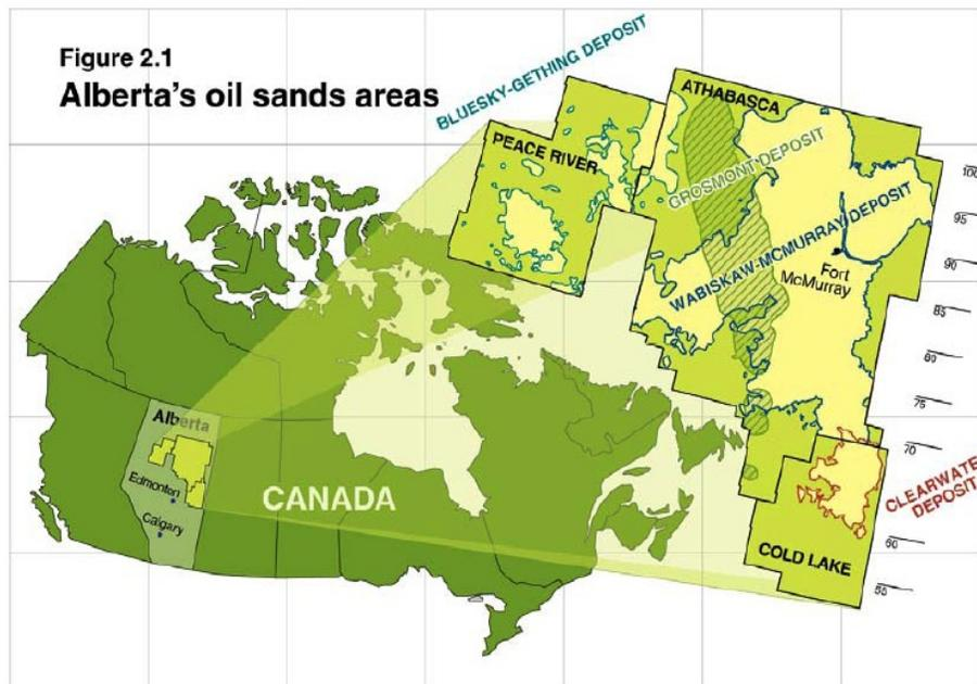
Alberta's crude bitumen resources are contained in sand (clastic) and carbonate formations in the three OSAs shown in Figure COS1. Contained within the OSAs are 15 major Oil Sands Deposits (OSDs), which designate the specific geological zones containing the oil sands. Each OSA contains a number of bitumen-bearing deposits.
