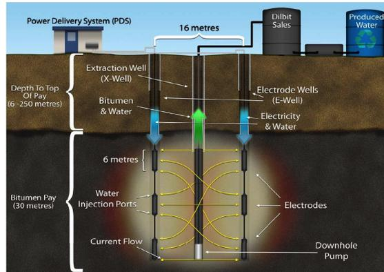
Shell has also tested electric heating at Peace River and has received approval for an electric heating experimental scheme in the Grosmont carbonates. The Shell process would heat the oil sands to high temperatures for long periods of time effectively coking the formation and producing upgraded or partially refined products. The process was originally developed for application to US oil shales.
