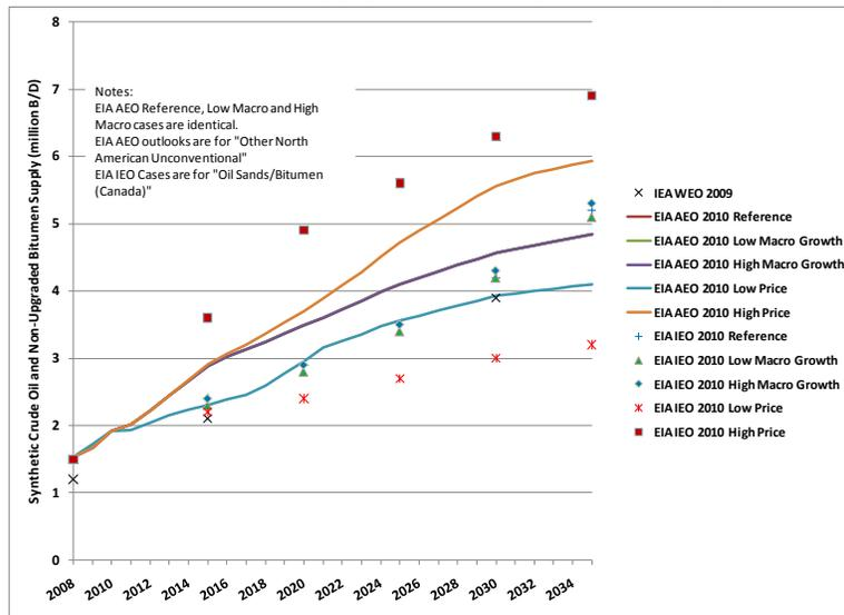
Based on our review of the available resources, the status of the industry and the challenges it faces, it is our view that the Canadian oil sands industry has the High potential to provide up to 6 MB/D of SCO and raw non-upgraded bitumen supply by 2035 as illustrated in Table COS3.
