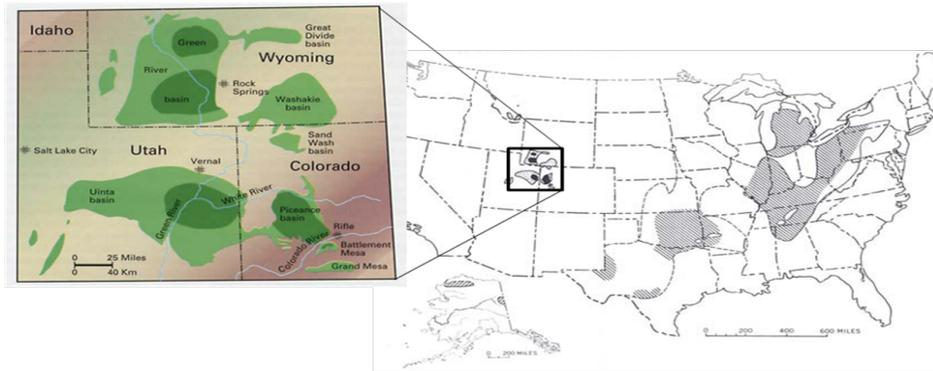
Because of thicknesses that can exceed 1000 feet, together with high richness, the Piceance Basin in Colorado is the most concentrated of these deposits with more than 1 BB of resource per square mile near the center of the Basin.
