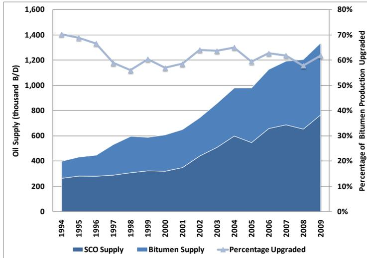
Note that some volumetric loss occurs due to upgrading – i.e., total bitumen production of 1,490,000 B/D resulted in the oil sands industry supplying 1,335,000 B/D of SCO and non-upgraded crude bitumen to downstream markets. Bitumen produced at all existing mining operations is normally upgraded, while most insitu bitumen production is not.
