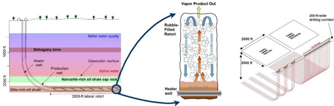
**Chevron** technology involves developing a series of fractures to increase the surface area of kerogen exposed, followed by use of a chemical process (as an alternative to high temperature) to convert the exposed kerogen to oil and gas. The proposed pilot will consist of four injectors and one producer.
