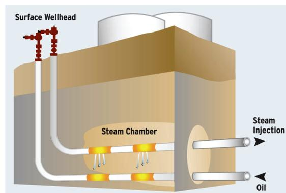
Operating mature SAGD projects reported average SORs of about 2.0-4.0 and average bitumen production rates of about 400-1,300 B/D per well-pair in 2009.<sup>63</sup> Recovery factors up to 65 percent of the bitumen in place within the project area are expected.
