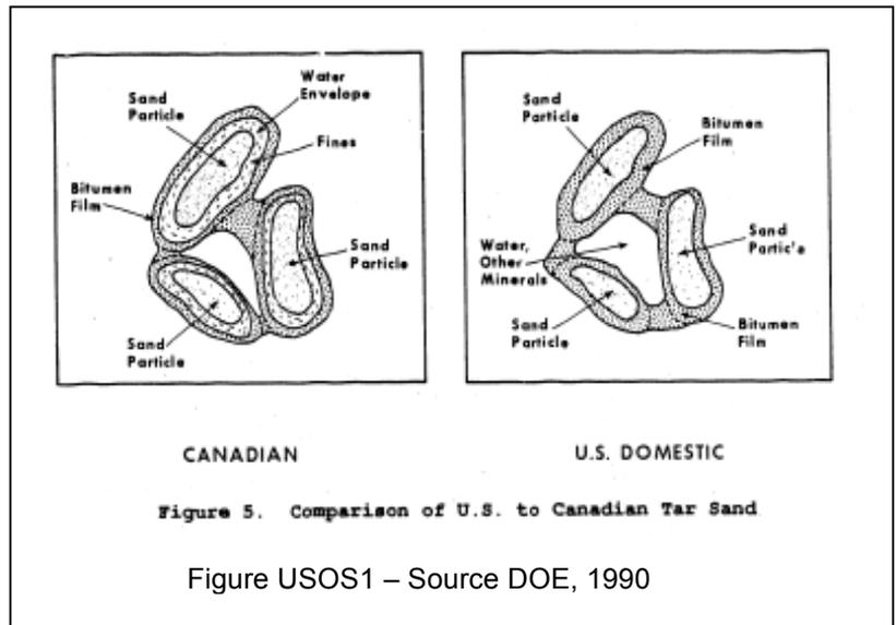
Cumulatively, the resultant differences are significant in that the traditional surface mineable extraction technique (the Clark Process) fundamentally relies on the film of connate water to achieve acceptable extraction levels. When engaged with Utah ores, extraction rates are typically around 80 percent giving unacceptable concentrations of residual bitumen in the discharged tailings and resultant poor economics.
