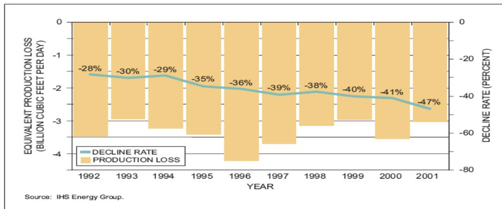
Figure S4-57. Gulf of Mexico Base Shelf - Decline Rate of Base Gas Production if No New Wells had been Drilled, and Equivalent Production Loss
