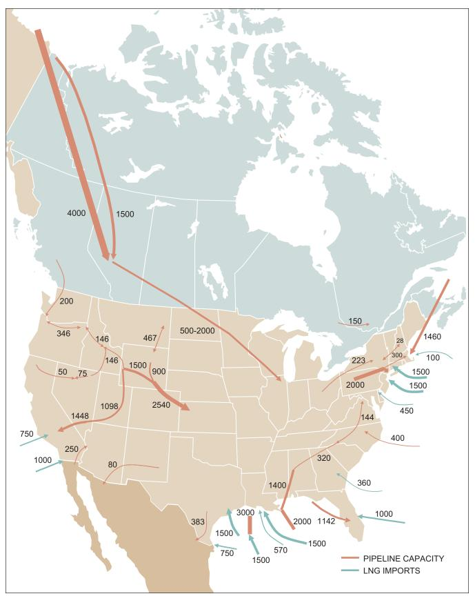
*Figure T-5.* New Pipeline and LNG Capacity Change from 2003 to 2025 in Balanced Future Scenario (Million Cubic Feet Per Day)
