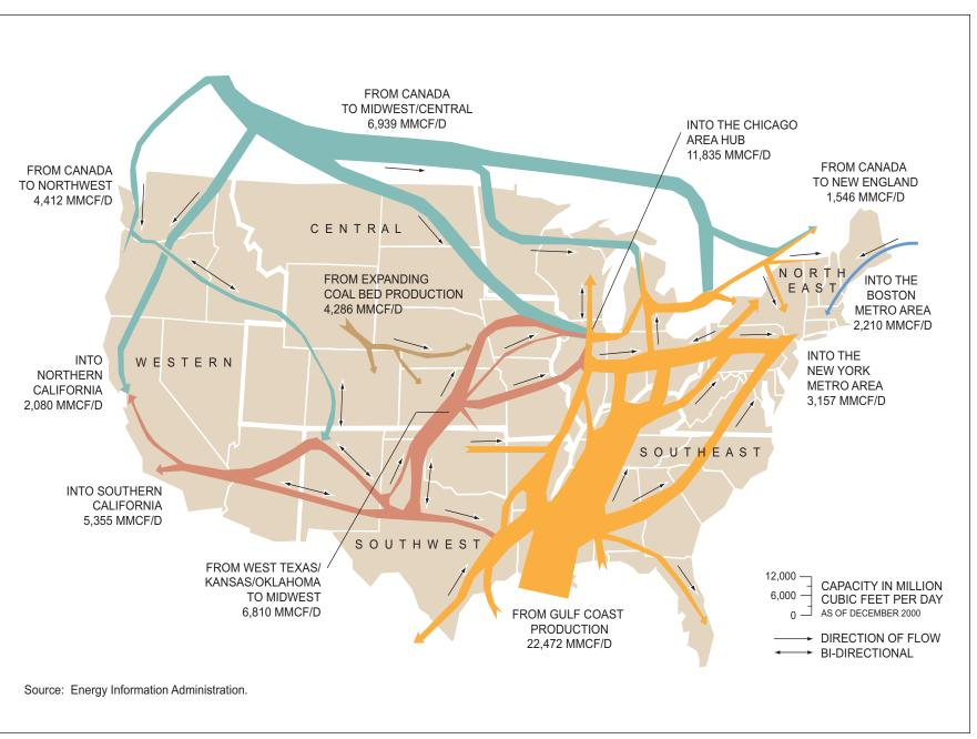
Figure L-15. U.S. Natural Gas Transportation Network
