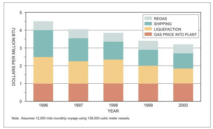
Figure L-4. Delivered Cost of LNG From a New Train Development
