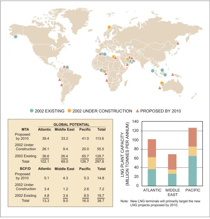
Figure L-11. Existing 2002, Under Construction, and Proposed LNG Liquefaction Capacity
