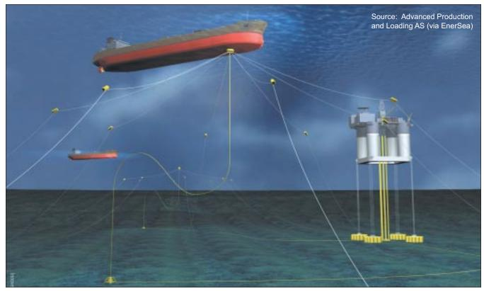
Figure D-3. CNG Carrier Loading Near Offshore Production Facilities
