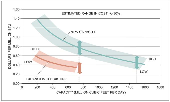
*Figure L-14. U.S. LNG Terminal Cost – Expansion and New Capacity*
