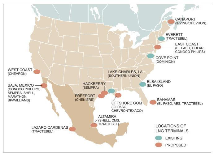
Figure L-17. Existing and Proposed North American LNG Import Terminals
