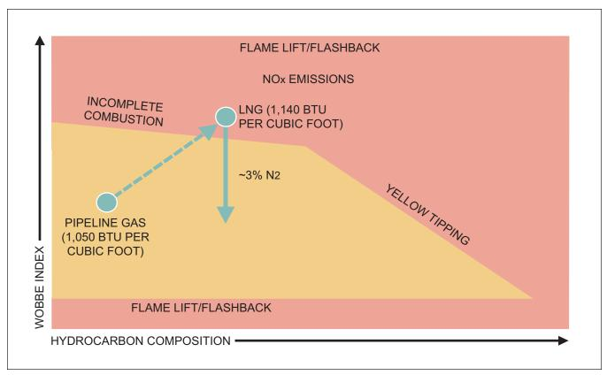
Figure E-3. Wobbe Index versus Hydrocarbon Composition
