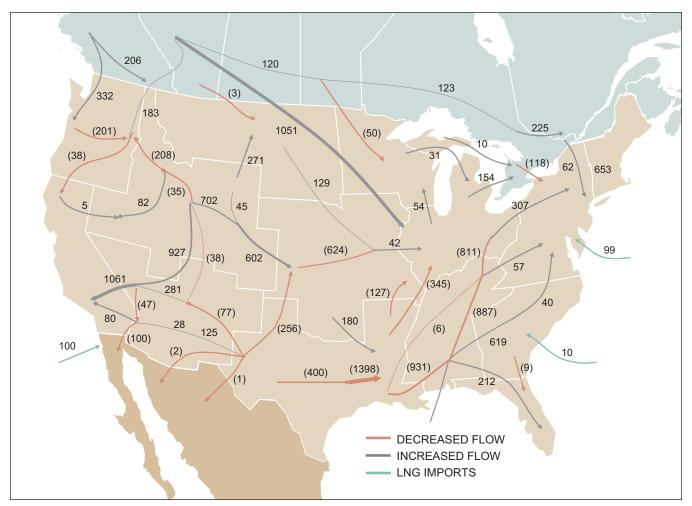
Figure T-7. Flow Change from 2010 to 2020 in Balanced Future Scenario (Million Cubic Feet per Day)
