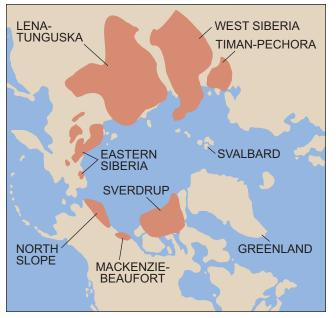
Figure S5-10. Arctic Basins – Areas of Known or Inferred Gas Hydrates
