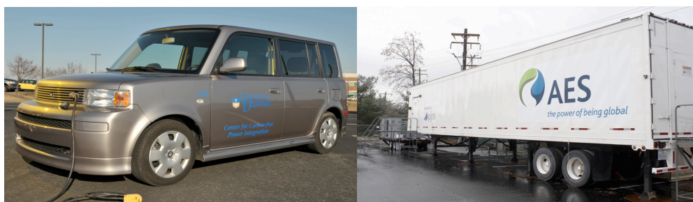
Figure 5: AC Propulsion eBox and AES 1 MW battery trailer array used to aggregate electric vehicles and bid their collective capacity into the market during V2G demonstration.
