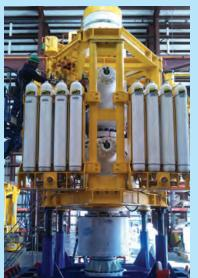
Photo: Trendsetter Engineering Inc. Subsea Isolation Device
