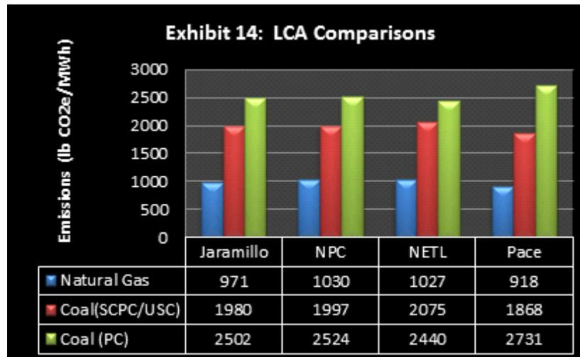
Figure 4. Comparison of emission estimates for natural gas and coal used as fuel for electric-power generation (Pace, 2009).
